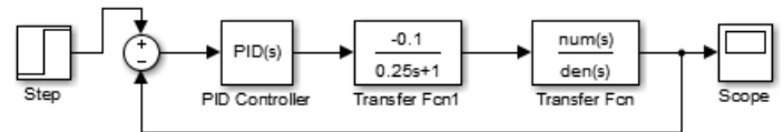
Fig.4. Block diagram of a UAV showing response of roll angle to elevon
