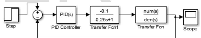
Fig.3. Block diagram of a UAV showing response of pitch angle to elevon
