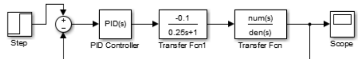
Fig.5. Block diagram of a UAV showing response of yaw angle to elevon
