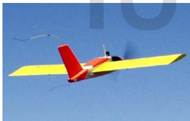
Fig.1. P15035 UAV, having only two independent elevon control surfaces.
